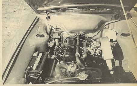
Engine is 1725 cc unit introduced CD Stromberg, as on Hillman GT. layout is excellent, finish well up.
